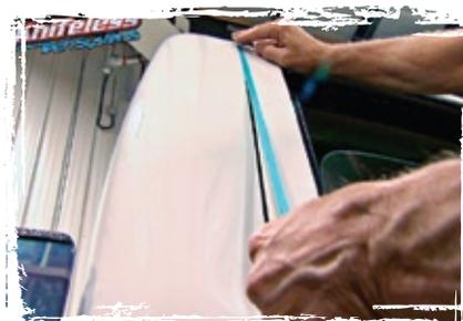
Knifeless Bridge tape is used here across a wide gap to avoid cutting or damaging rubber seals. With Knifeless Bridge tape there's no need to remove seals.
