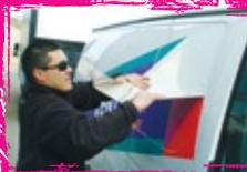
3. Lift an edge and pull. The vinyl will come off in larger pieces because it has been rejuvenated. Most of the adhesive should come with the vinyl!
